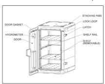
These cabinets have two door latches on the right side and hinges on the left. Leave space in front for the door to swing open. Place desiccant cartridges in the bottom of the cabinet and place the shelves into the cabinet starting at the bottom. Shelves must be angled 45 degrees to fit through the door opening.
