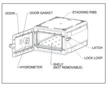
The cabinet should be placed on a horizontal surface with the door latch on the right. The space in front of the cabinet should be left clear to provide space for door opening.
