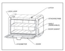
This cabinet is the same size as the 4.0 vertical but is wider and lower than the vertical cabinet. The door is hinged at the bottom and has two latches at the top. Two removable shelves are included. With the two shelves in place, the distance between the shelves is 110 mm (4-3/8") minimum.
