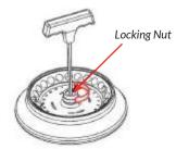
Load the Rotor Onto the Shaft
