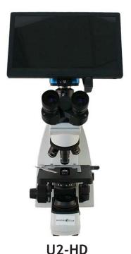
High definition HD camera and 12" HD monitor for fast frame rate. Capture images to SD card or computer.
