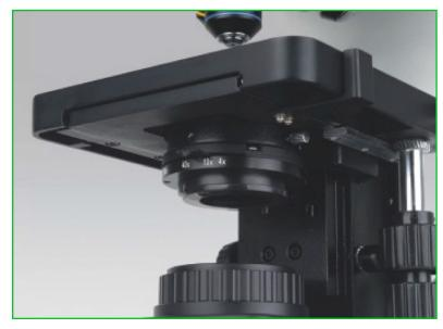
Fixed Koehler illumination with Infinity Corrected optics ensure high resolution, sharp and clear images.
