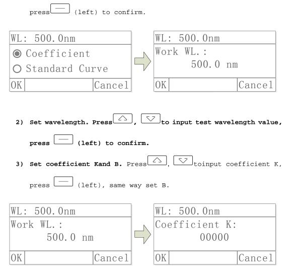
Method 2: Establish Standard Curve by using Standard Samples
