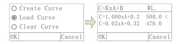
Press (left)to enter the test mode after building or loading standard curve.
